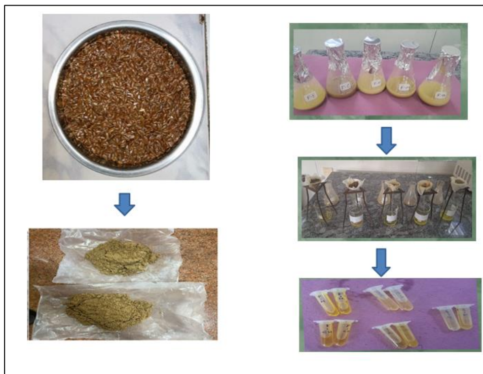
Fig.1 Stepwise preparation of flaxseed powder and solvent extraction process. (A) Whole flax seeds, (B) ground flaxseed powder, (C) maceration of plant material with solvent, (D) filtration of extract and (E) obtained clear filtrates for further analysis.
